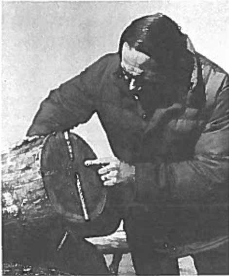
Figure 2. Dr. Labosky examines a typical pile of dead 3-year-old oak logs showing excessive end checks.
